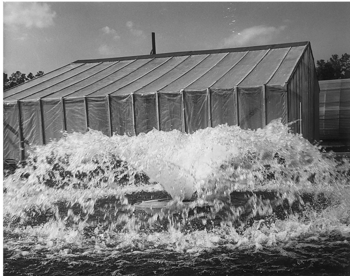
Fig. 1. A vertical pump aerator.
